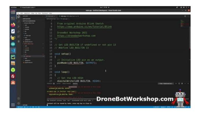
The error is produced because the constant LED\_BUILTIN is not predefined for the ESP32. In addition, the ESP32 board uses a different pin for the built-in LED.
