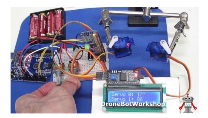
Try out the project, you should be able to move both servo motors and observe their position on the display.
